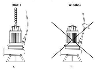
Figure 1. Lifting the pump property
