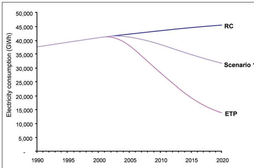
Figure 2. Electricity consumption by circulation pumps in the EU according to current (RC) and potential consumption scenarios<sup>6</sup> (reproduced courtesy of Grundfos A/S).
