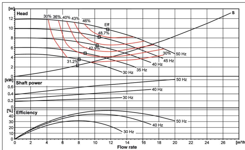
Figure 3. The reference single pump performance curve for the variable-speed circulation pump used in the study.
