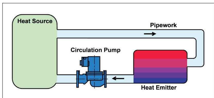
Figure 1. Simplified diagram of a typical heating system with a circulation pump.
